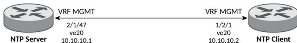
FIGURE 3 Use Case 1: Management VRF Forwarding with One Client and One Server on VE
